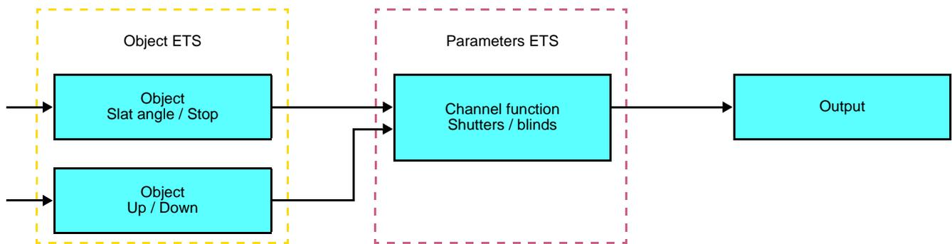
This function controls shutters or blinds using two push buttons (Input). One button for Up and one button for down. The function transmit the **Up / Down** object (long key press) and the **Slat angle adjustment / Stop** object (short key press).
